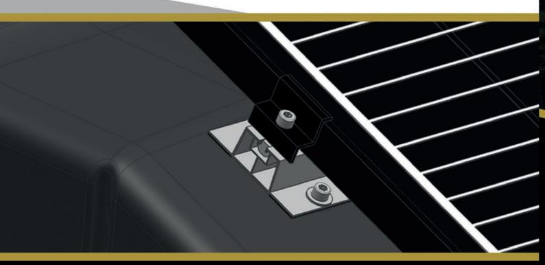
The GRAM-BOX system is adapted to mount all photovoltaic panels available on the market, regardless of the type, dimensions and power. Thanks to its features, the mounting can be performed much faster, and its time reduced by up to 80% compared to the existing solutions. The mounting of panels can be performed even by a single installer and the cost of transport to the place of installation is much cheaper.
